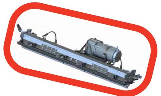
Initial install requires about 4-8 hours to modify the existing gate box to the rotary drum mechanism and its motor. This also accounts for the installation of the cockpit control box and wire harness. After the initial install, normal operation switching between the Meterate arrangement back to standard can take as little as 45 minutes.
